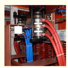
, 4000KVA Induction Furnace Power Supply
